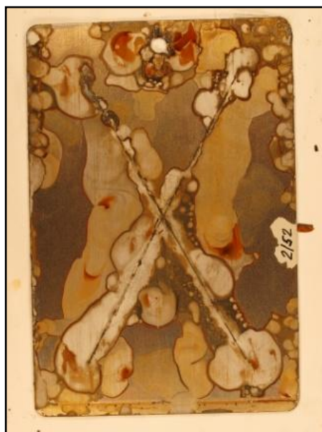
Fig. 1 Evaluation of delamination according to ČSN EN ISO 4628-8 – 1000h, IV - Ferroclean+E-CLPS, Degree: 5 – very large
