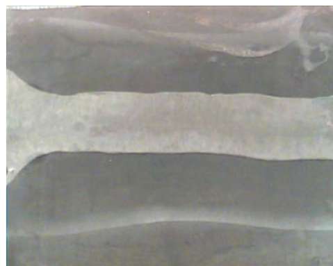
Fig. 3. Rail weld joint, outside of damage
