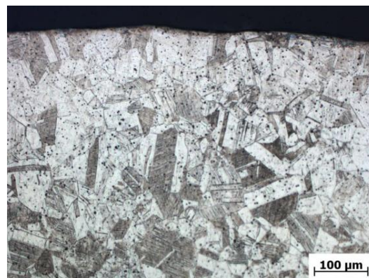
Fig. 1. Microstructure of AISI 316Ti steel, electrolytic etching.
