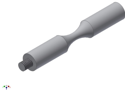
Fig. 1. Specimen for measurement internal friction
