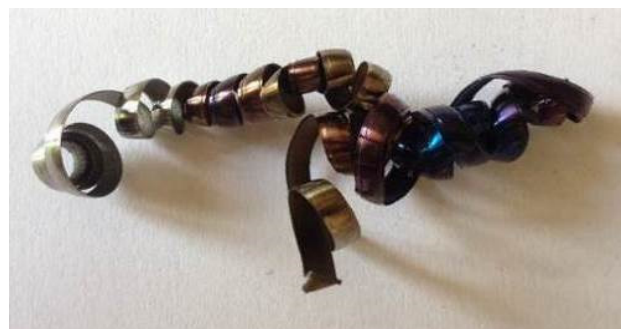
Fig. 10. Chip coloured due to cutting temperature
